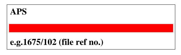
The lettering on the label may be printed or written. If written, a thick black felt marker of a kind suitable for cold store use should be used. The letters and numbers should be between 1 and 1.5 cm in height.
