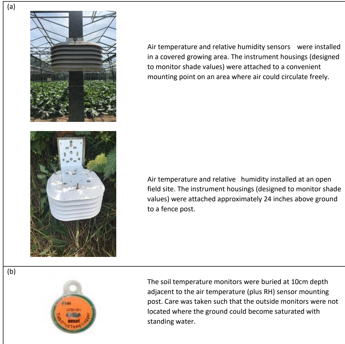
Figure 2. Methods of deployment for (a) air temperature and relative humidity sensors and (b) soil temperature sensors.
