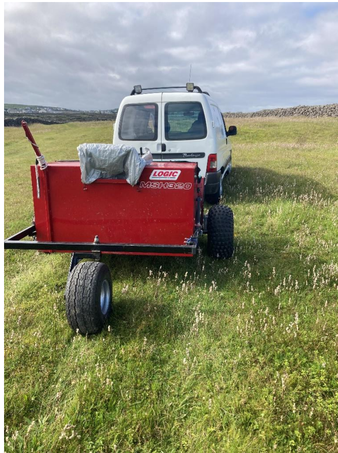
Fig.9 Gathering Wildflower Seed, machine drawn brush harvester
