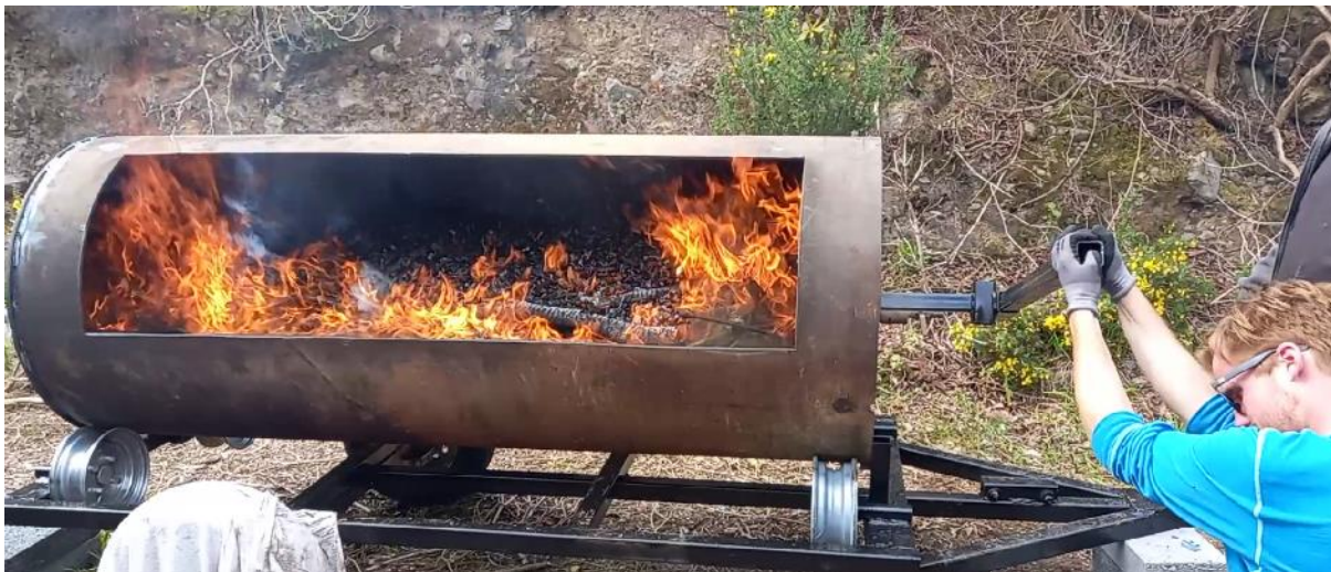
Figure 24 The RoCC Kiln built by the NCLLAES scheme for making biochar.
