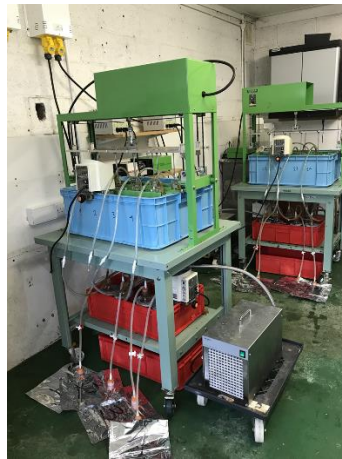
Figure 11: RUSITEC Machine used to analyse rumen methane emissions
