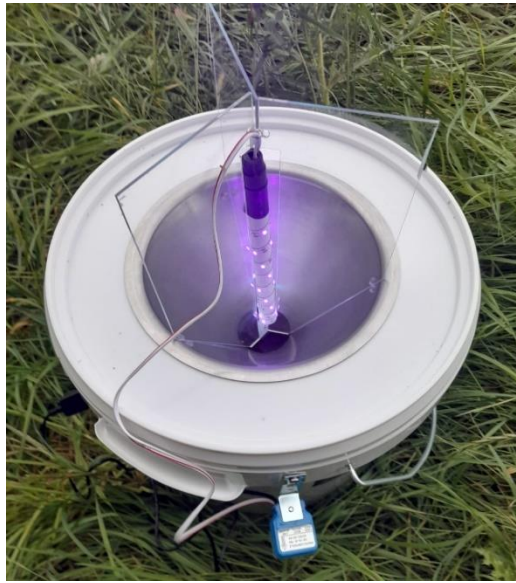
Figure 2: The assembled LedEmmer trap with illuminated LED strip.
