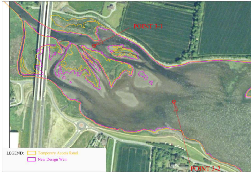
Malahide Viaduct Reinstatement - Water surface comparison at spring low
